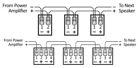
Typical 70V/100V installation wiring method
